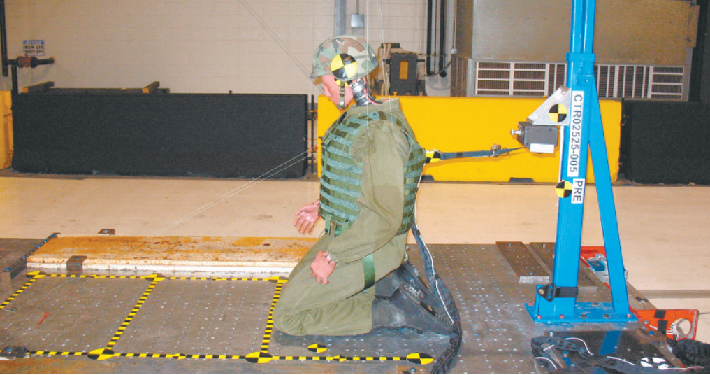
Wolf Technical's energy-absorbing system restrains air crew members slowly rather than jerking them to a stop.
